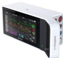
The [Philips IntelliVue X3](#) is a portable and compact patient monitor, designed to allow hospital staff to continuously monitor their patients and move safely through hospitals. The device acts as a multi-measurement module when connected to a bedside monitor, and, once detached, functions as a transport monitor.
